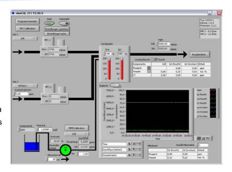
viewCAL enables the calibration of each gas flow controller and the liquid flow sensor. The characteristic of the flow controllers will be fitted by means of a polynomial (3<sup>rd</sup> order) function), which increases the accuracy enormously.
