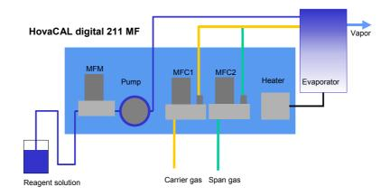
A peristaltic pump is used for dosing the reagent solution or pure water in the evaporator. The quick response time of the sensor enables to operate the device self regulating. I.e. the set point concentration of water vapor or a reagent component will be achieved automatically.
